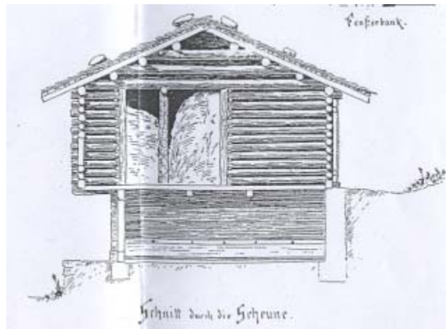
Cantilevered Forebay- with Bank on Back side
